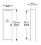
Fabricated from metal, and powdercoated, to withstand the external elements, the cabinet is mounted at the ground level for easy access for emergency and maintenance purposes.
